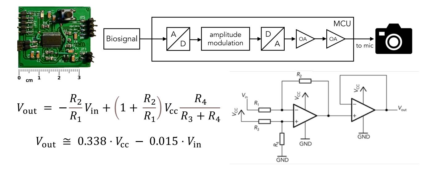
During our measurements, we used as a PPGI sensor a Canon 550D DSLR camera with modified firmware, which allowed us recording raw video in MLV format with a sampling rate of 15 Hz. As sensors of the reference signals, we used a SparkFun Electronics contact PPG sensor placed on the index finger and an ECG analog front-end based on AD8232 (Analog Devices) again on a prototype board from SparkFun Electronics. The ECG signal was recorded from the Einthoven lead I.
