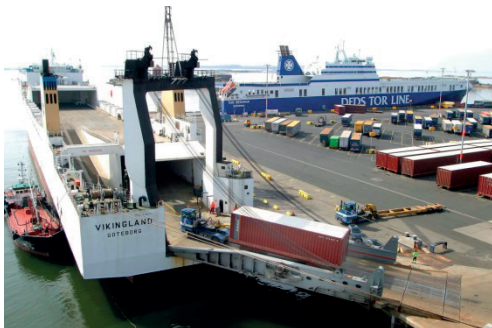
Fig. 3 Ro-Ro transshipment process [7]
