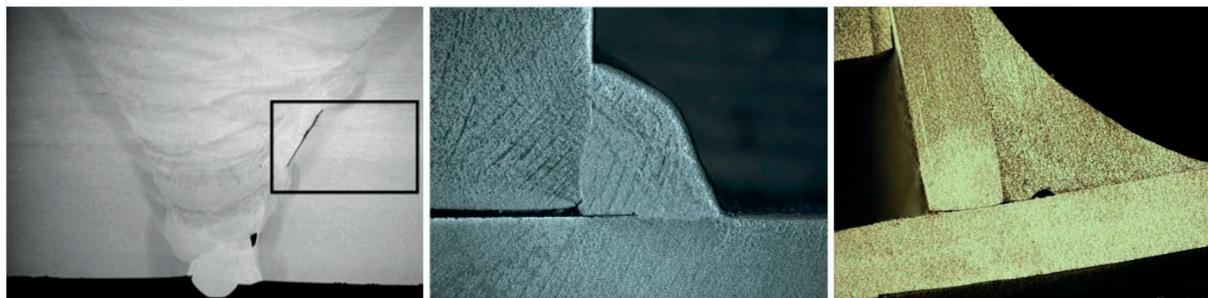
Fig. 2 Lack of fusion and penetration [4]
