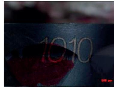
a) sharp cutting insert, VB = 0.05 mm
