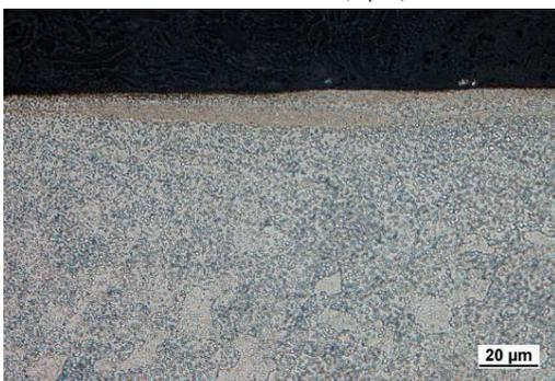
Fig. 6 Microstructure of milled surface, VB = 0.8 mm, HAZ (5.5 μm)
