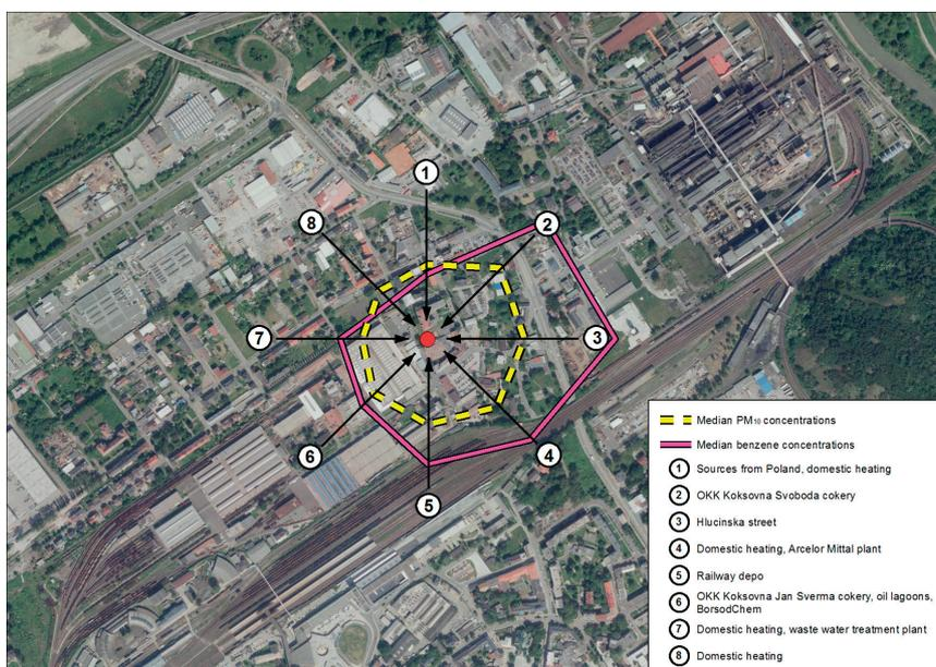
Fig. 1 Location of the monitoring station, pollution sources direction and median of  $\text{PM}_{10}$  and benzene concentration [2]
