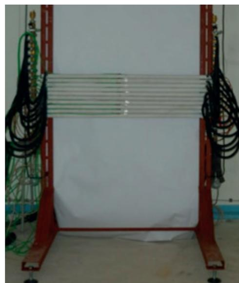
Fig. 3 Arrangement of pipes in a thermostatic chamber at axial distance of pipes  $1D$  [6]
