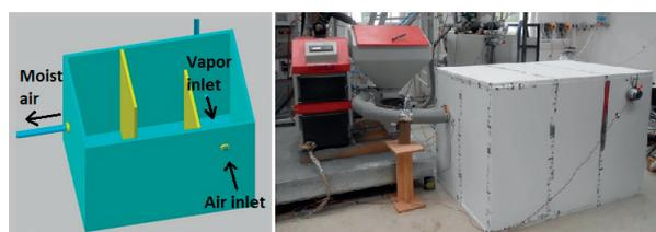
Fig. 3 The principle of combustion air humidification
