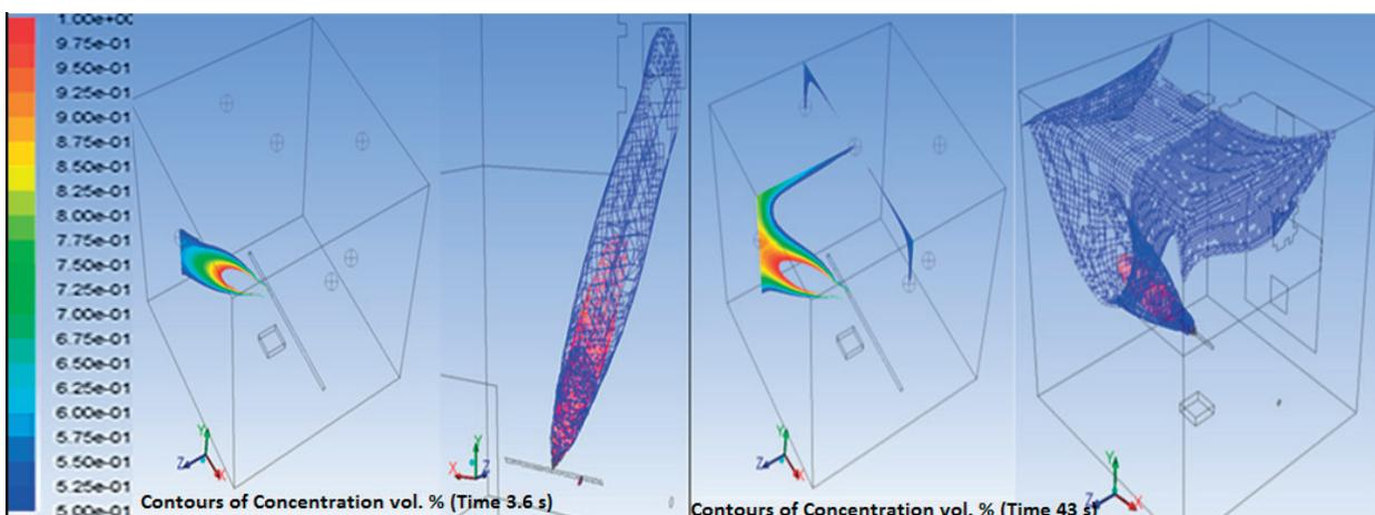
Fig. 8 Local concentrations (0.5 vol. %) during reaction of the sensors Nos. 1 (on the left) and 2, 5 and 6 (on the right)
