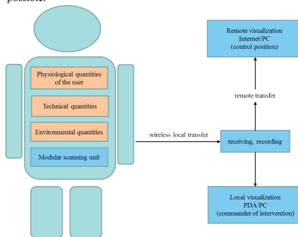
Fig. 1 Principles of the FlexiGuard surveillance system function
