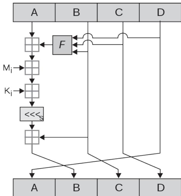
Fig. 2 An MD5 encryption round Source: [9]
