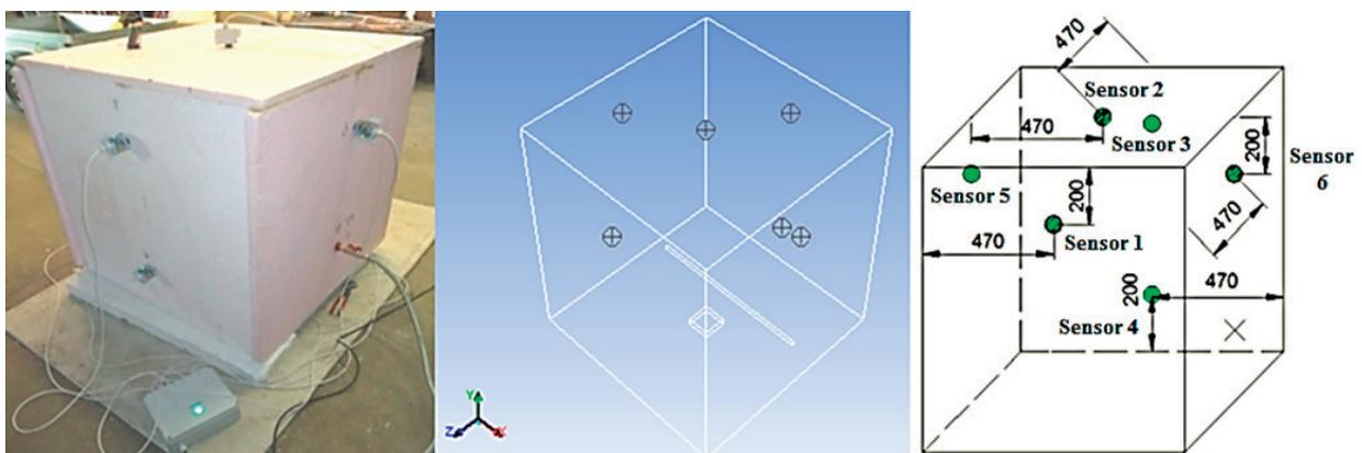
Fig. 5 Position of detectors and of tracepoints (mm)
