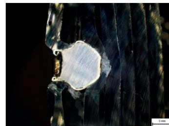
Fig.2 Cross-section of bullet in polycarbonate board [6]
