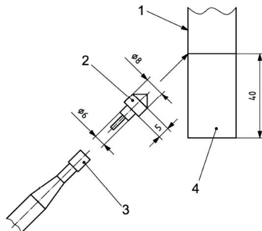
Fig. 5 The scheme of the flame impact on the surface of test specimen (1 - specimen surface, 2 - spacer, 3 - gas burner, 4 - test specimen) (see [6])
