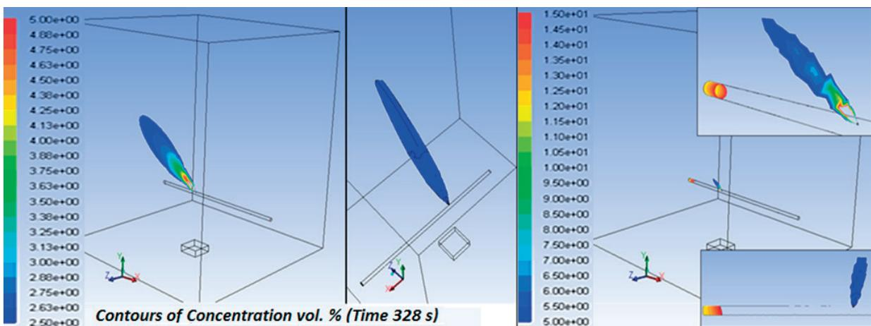
Fig. 13 Dangerous (on the left) and explosive (on the right) concentration right before the end of experiment
