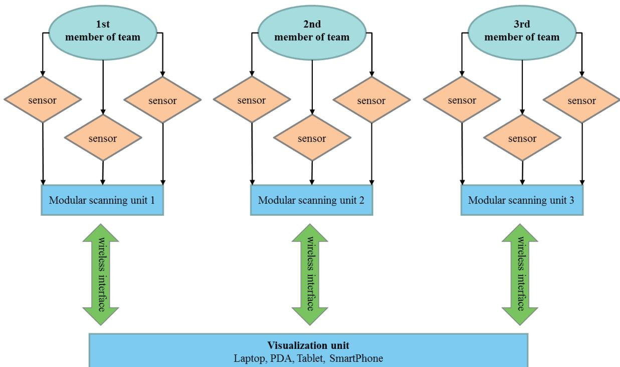
Fig. 2 Modular concept of the FlexiGuard surveillance system
