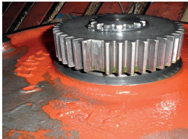
Fig. 6 Sun gear with one missing tooth
