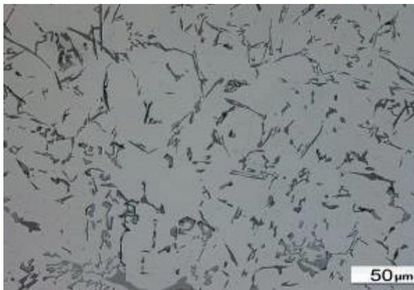
Mag. 200 x and 500x, etching 20ml H<sub>2</sub>SO<sub>4</sub> + 100ml H<sub>2</sub>O
