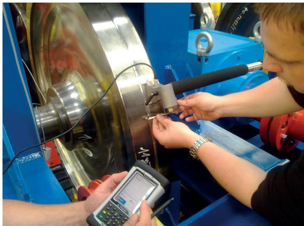
Fig. 11 Rails tread measurement with MiniProf device
