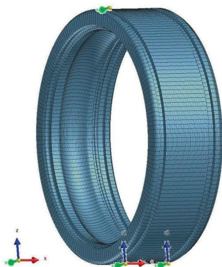
Fig. 4 Scheme of the outer ring in the SYSWELD software
