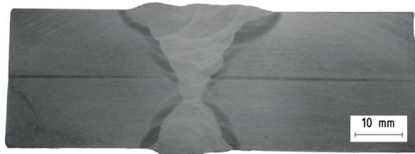
Fig. 6 Macrophotography of welded joint, etch. 5% Nital
