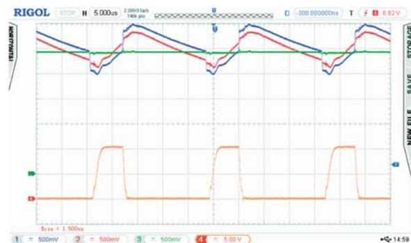
Fig. 13 Measurement signal of the LEM current sensor (red), hysteresis (blue), offset voltage (green) and gate-source voltage (orange)
