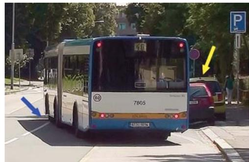
Fig. 12 Exiting the bus from the bus stop influenced by parallel parking places (yellow arrows) and subsequent driving into opposite direction (blue arrows); the left photograph from the point III (see VIDEO 06 [8]) and the right photograph from the point II (see VIDEO 07 [8])
