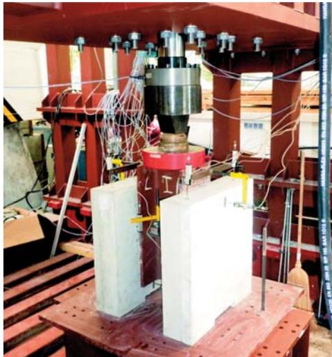
Fig. 2 Configuration of the push-out test
