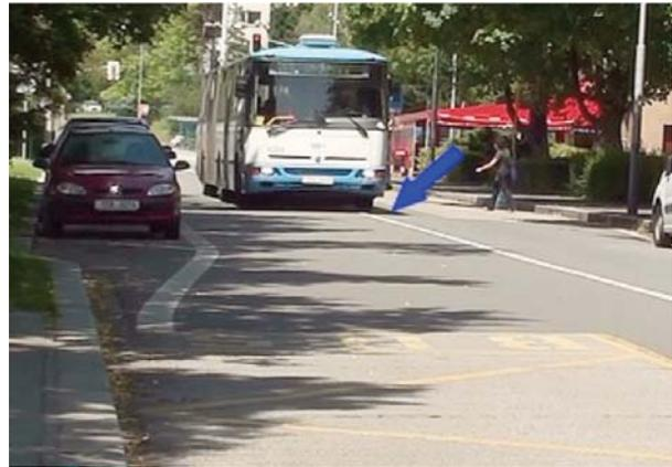
Fig. 11 Crossing the bus into opposite direction due to inadequate width proportions (point I; see VIDEO 04 and VIDEO 05 [8])
