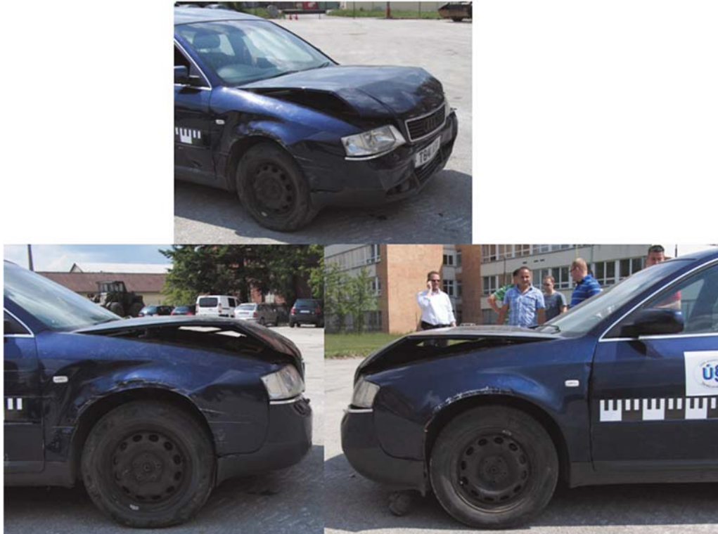
Fig. 8 Damage of the car Audi (EES = 18 km/h)
