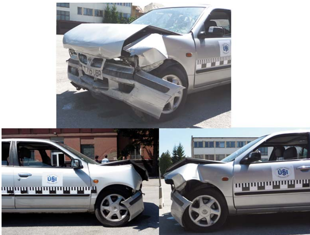
Fig. 4 Damage of the car Nissan Primera (EES = 54 km/h)
