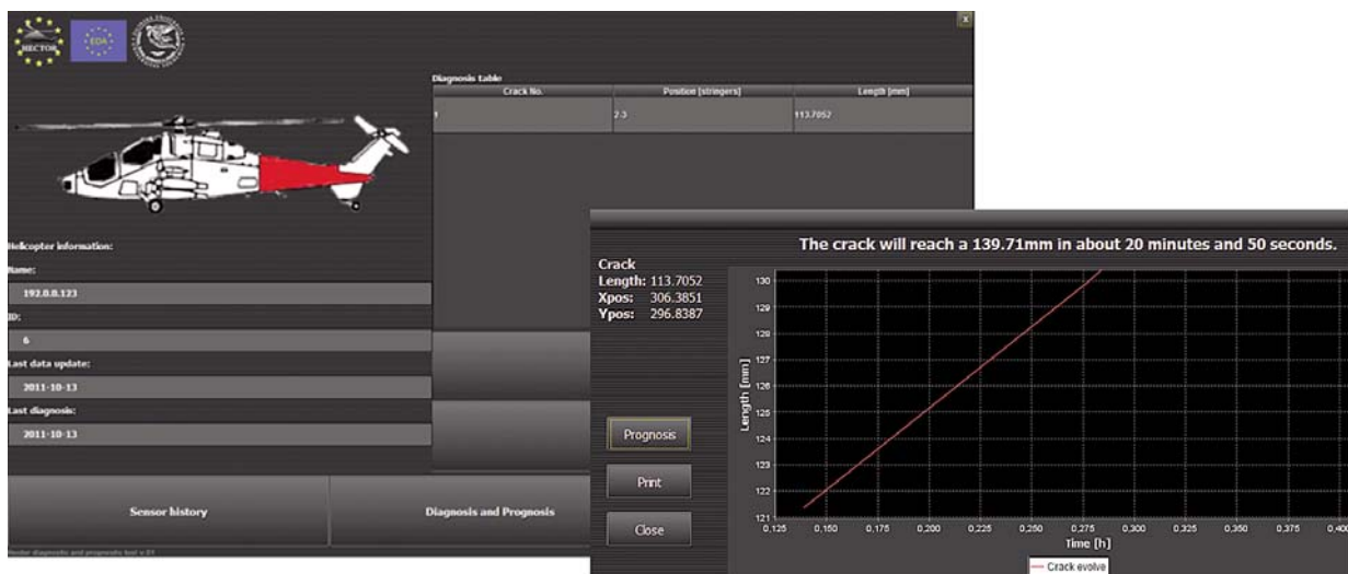
Fig. 8 Graphic user interface for Maintenance Unit
