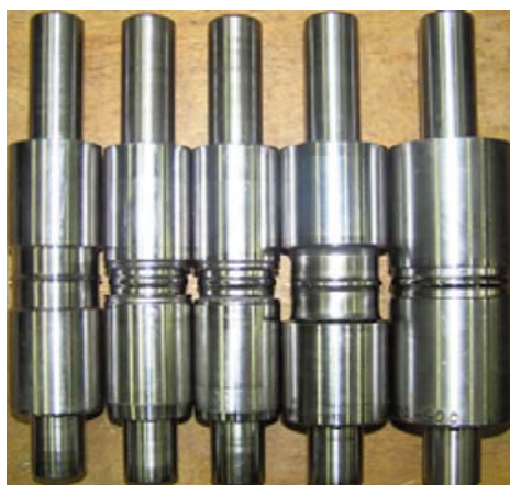
Fig. 6 Thorns on rolling bearing rings
