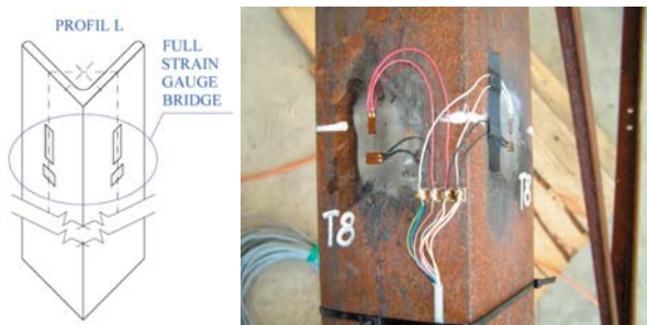
Fig. 2 A position of strain gauges on the chosen place of L-profile
