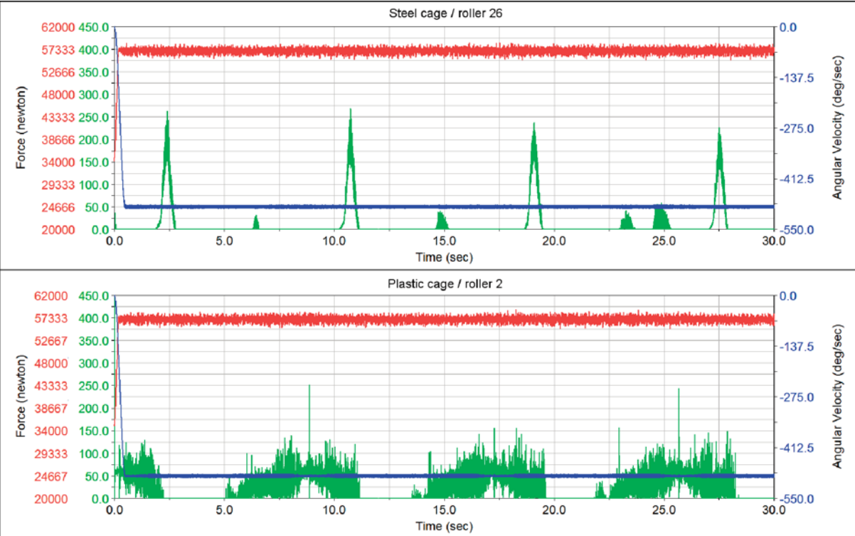
Fig. 3 Force interaction between inner ring and rollers (red lines), force interaction between cage and rollers (green lines) and angular velocity of rollers.
