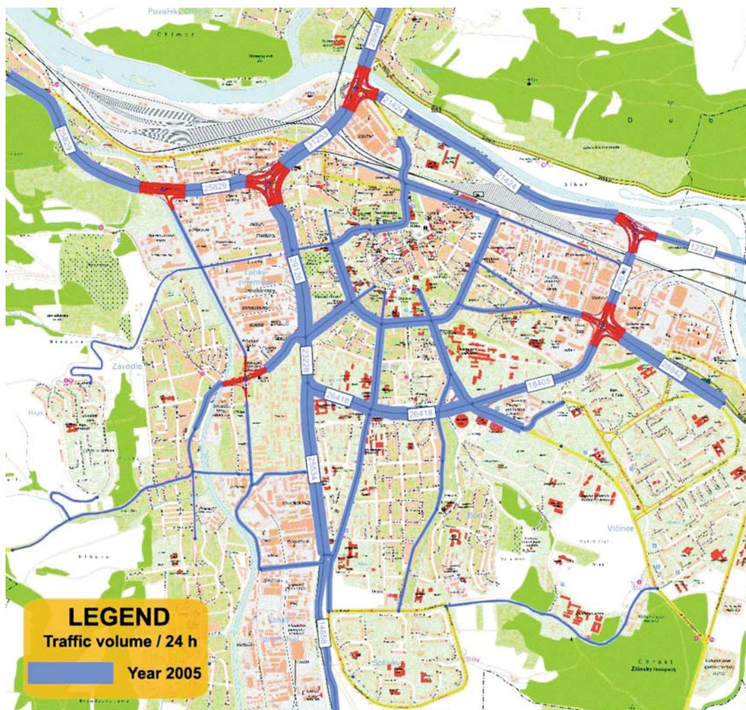
Fig. 7 Traffic loading of Žilina road network
