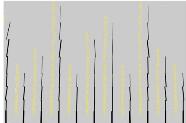
Fig. 11a) Crack propagation - experiment, ATENA - the 11. load step
