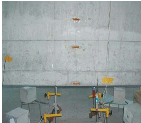
Fig. 11a) Crack propagation - experiment, ATENA - the 11. load step
