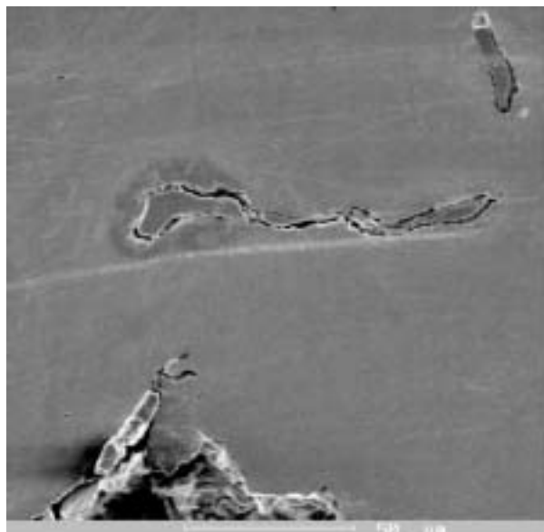
Fig. 15 The separation of an inclusion from basic material, REM
