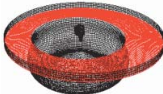
Fig. 4 Surface grid of combustion chamber without the engine head grid
