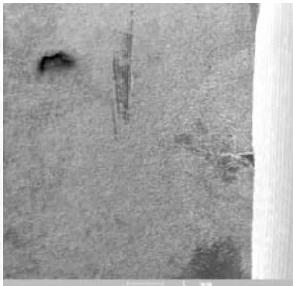
Fig. 23 The beginning of the crack growth – one of the sources, REM
